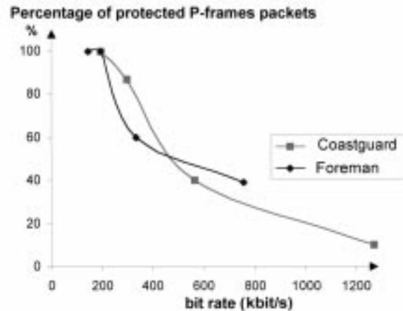
Fig. 4. Percentage of protected P-packets by the UPP mechanism. (The bit-rate range for the two sequences is different since the simulation was based on constant QP rate-control).
