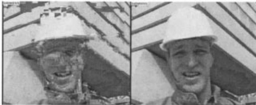
Fig. 5. Frame #14 from the *Foreman* sequence coded at 332 kbit/s, with NS QP = 6 (left) and FGS with UPP (right) both after one packet-loss event. For FGS, the entire enhancement-layer of this frame is lost (i.e., a worst case scenario), and the image quality is reduced to the base-layer quality. However, in the NS case, due to a packet-loss in a previous frame, the error propagated, leading to a distorted image.
