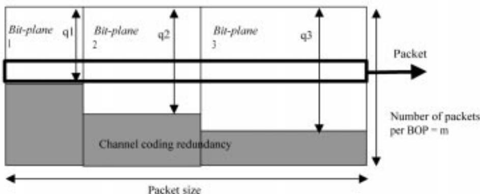
Fig. 11. Transmission of an FGS stream containing  $n = 3$  bit-planes.
