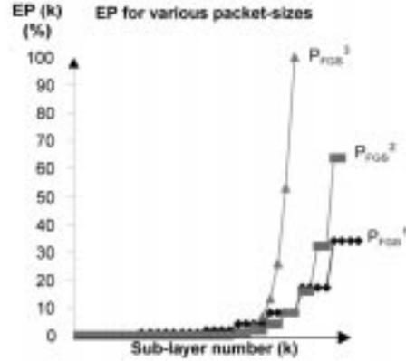
Fig. 7. Effective packet-loss ratios of each sublayer  $E(k)$  dependent on the packet-size.
