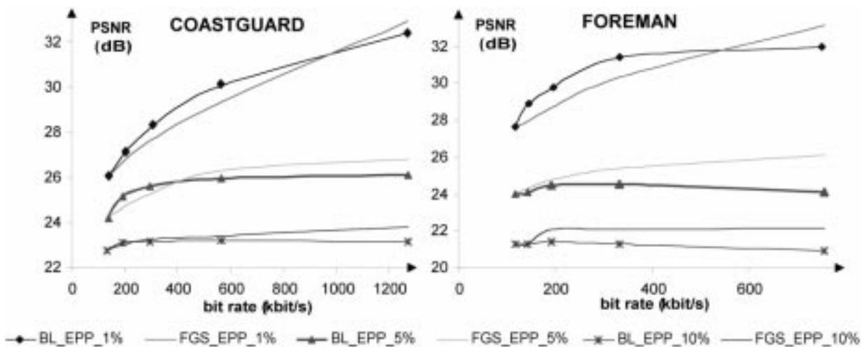
Fig. 2. Packet-loss resilience of NS and FGS under EPP.
