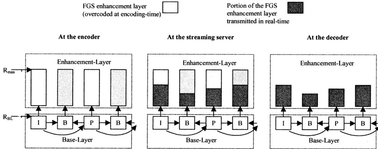
Fig. 1. FGS scalability structure at the encoder, streaming server, and decoder for a typical Internet streaming application.
