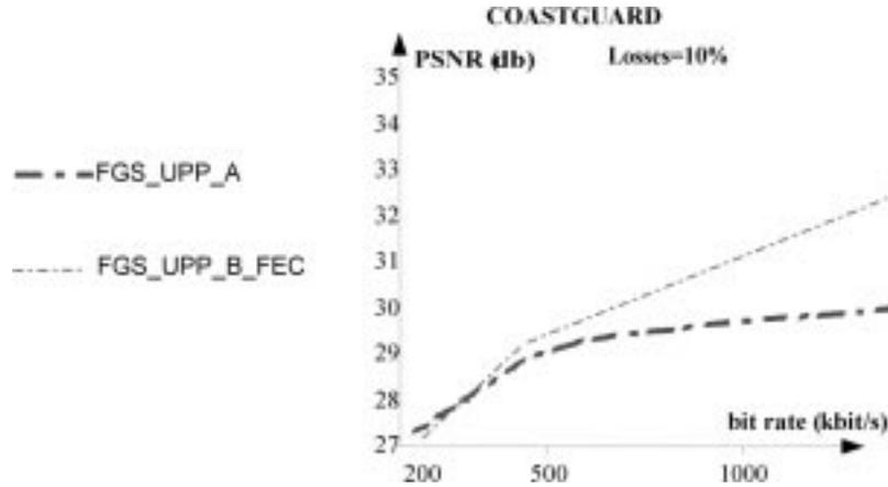
Fig. 12. Performance results of the UPP\_B FGLP protection strategy using FEC for its implementation. In the UPP\_A case, there is no protection for the enhancement-layer.
