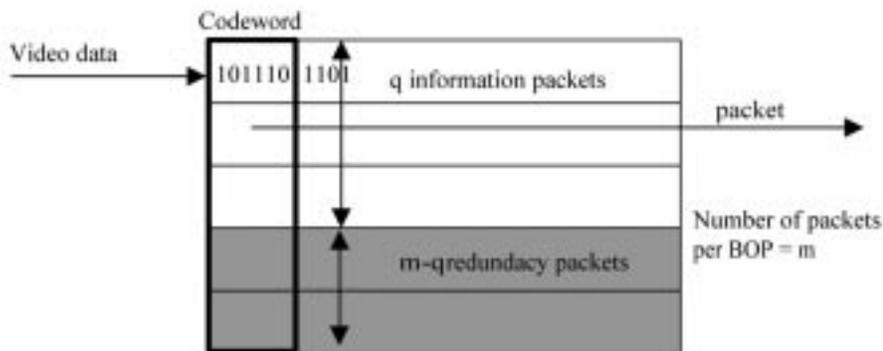
Fig. 10. FEC across packets according to [7], [26]. The video bitstream is written line-wise into  $q$ -packets. Additionally  $m - q$  packets are generated by forming codewords column-wise. All  $m$  packets together form one BOP.
