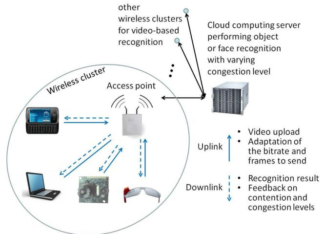
**Fig. 1.** Illustration of object or face recognition via adaptive wireless video transport to a remote computing server.
