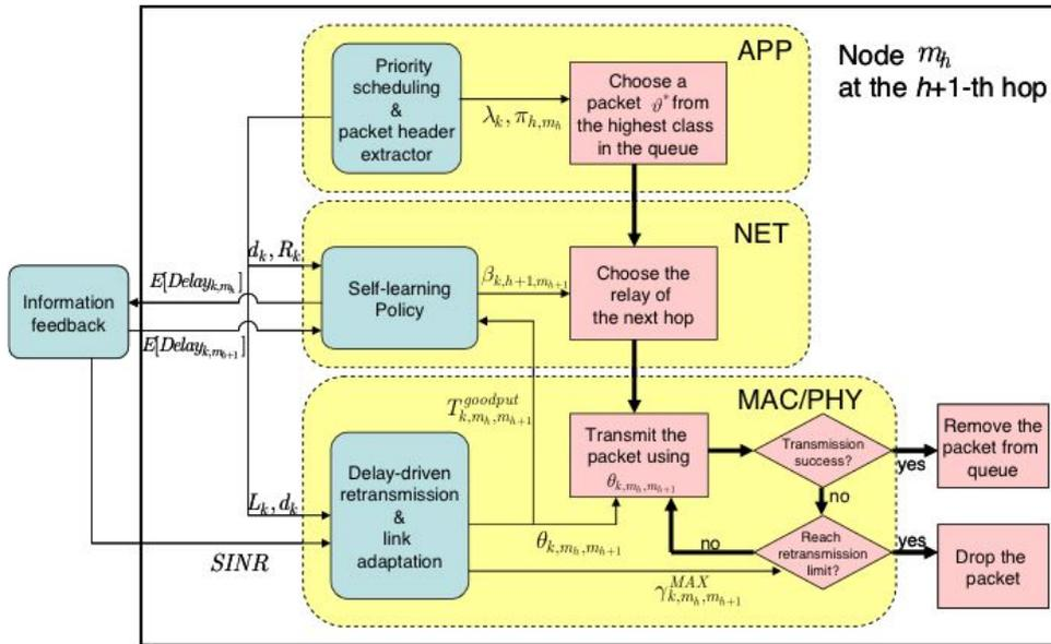
Fig. 2. Integrated block diagram of the proposed distributed per-packet algorithm.
