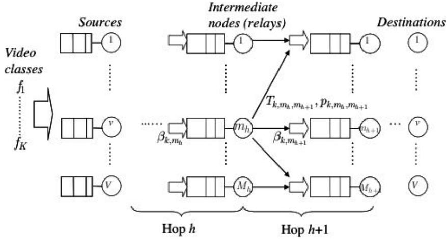
Fig. 1. The multi-hop overlay network model with  $V$  video users and  $K$  priority classes.
