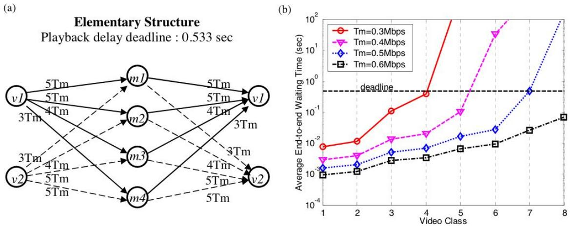
Fig. 5. (a) Network settings of the elementary structure. (b) Analytical average end-to-end waiting time of the 8 video classes.
