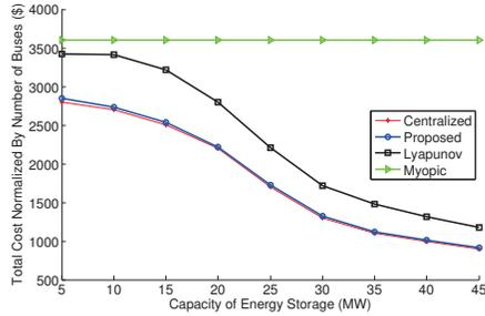
Fig. 3. The normalized hourly total cost versus the capacity of the energy storage.
