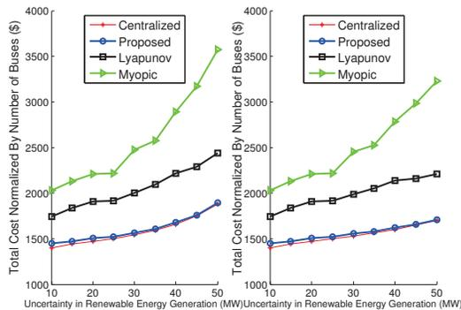
Fig. 4. The normalized hourly total cost versus the uncertainty in renewable energy generation. The aggregators have energy storage of capacity 25 MW and 50 MW in the left and right plots, respectively.
