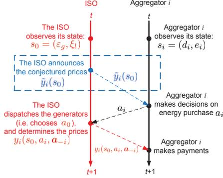
Fig. 2. Illustration of the entities' decision making and information exchange. The action and the message exchange in the dashed box are related to the conjectured prices proposed in the design framework in Sec. III.
