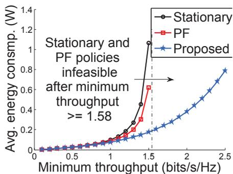
Fig. 6. Comparisons of energy efficiency under different minimum throughput requirements.
