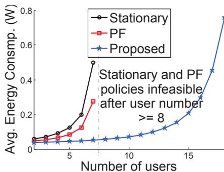
Fig. 5. Comparisons of energy efficiency under different numbers of users.
