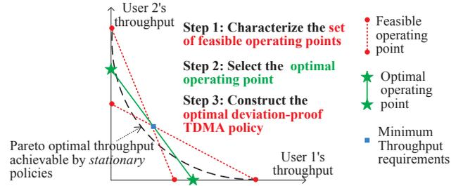
Fig. 2. The design framework to solve the policy design problem. The feasible operating points lie in different hyperplanes (red dash lines) that go through the vector of minimum throughput requirements (the blue square).
