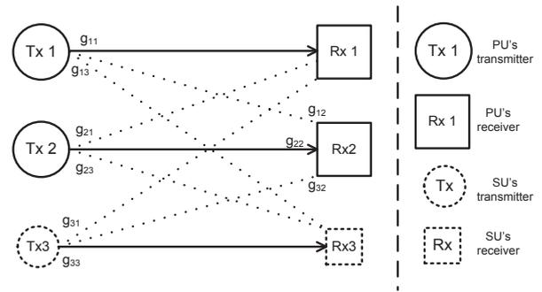
Fig. 1. An example system model with two primary users (transmitter-receiver pairs 1 and 2) and a secondary user (transmitter-receiver pair 3). The solid line represents a link for intended data transmission, and the dotted line represents the interference from another user.
