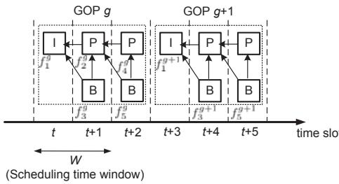
**Fig. 1.** Illustration of GOP (group of pictures), DU (data unit), and packet scheduling. Since the scheduling time window is  $W = 2$ , the contexts in different time slots are  $C_t = \{f_1^g, f_2^g, f_3^g\}$ ,  $C_{t+1} = \{f_2^g, f_3^g, f_4^g, f_5^g\}$ ,  $C_{t+2} = \{f_4^g, f_5^g, f_1^{g+1}\}$ ,  $C_{t+3} = \{f_1^{g+1}, f_2^{g+1}, f_3^{g+1}\}$ , and so on.
